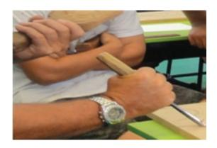
The tools used is a haehae chisel and a mallet on MDF wood. In Aotearoa conventional kaiwhakairo use the chisel with the mallet. Other cultures use different techniques for carving.
