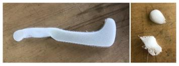
Despite this failure, I was still able to use the partially printed model to test the ease of raft / support removal, particularly on the curved handle. I found this to be surprisingly effective with the right tools, and left a very nice bottom surface as seen above right (handle segment at top of image, removed waste at bottom of image).
