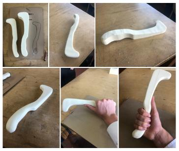
This is the finished model of the prototype, as well as some close ups of the handle shaping, which I took a lot more care in this time: I went for smoother curves overall, with a slightly deeper back edge curve, and a less prominent front edge grip curve. I also made the handle bigger and more raised, with a greater taper to balance the stick out more, along with a rounded edge on the bottom curve of the handle to help with grip purchase.
