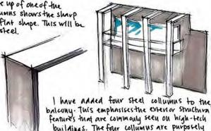
I have added four steel columns to the balcony. This emphasises the exterior structural features that are commonly seen on high-tech buildings. The four columns are purposefully similar to the main side of the building—this makes the side look balanced. The shadow of the columns also could provide shade for girls who are up on the balcony. I may need to adjust or refine them because it could feel cage-like and not as open as I originally intended.
