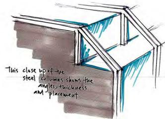
This close up of the steel columns shows the angles, thickness and placement.
