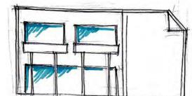
This is the front on view of the senior common room. I have made the steel columns run over the roof. This building so the structural detail flows better. The columns go over the roof and to the other side of the building—as the picture on the right top hand corner shows! I have made my senior common room suited to my chosen architectural movement. I was inspired by the look of the Centre Pompidou, although I simplified the structural look and kept the basic concept of it.
