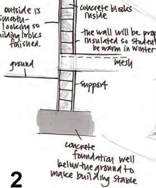
Two of my building's walls will be load bearing concrete walls. It is appropriate because there are no windows at these faces so installation will be easy. The concrete will also go into the steel aesthetically because the concrete will be exposed from the outside. It has raw, exposed materials on the outside.
