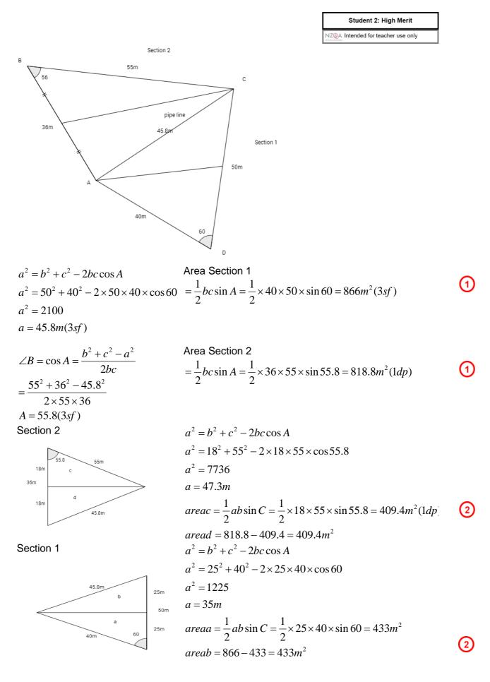
If you split section 1 between CD and join up with A and section 2 between AB and join up with C you can create 4 sections all over  $400m^2$ .
