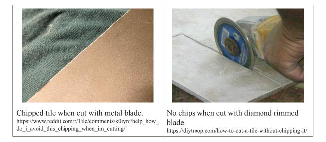
A diamond blade is less malleable than a metal blade.
