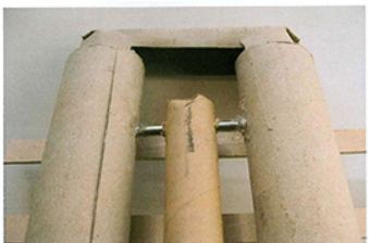
THE RESTING ARM WILL SWIVELL ON A BAR THAT WILL ACT AS THE PIVOT POINT.
