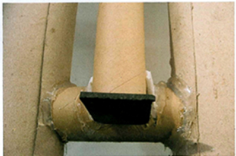
THE TWO WHITE PIECES OF PERSPECTS REPRESENT THE CLIP THAT THE RESTING ARM WILL CLIP INTO WHEN NOT IN USE.
