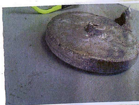
Open cast flywheel All the impurities are on the top layer of the cast, which you have to machine off.
