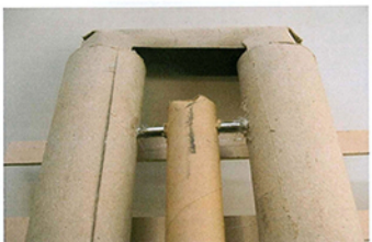
THE RESTING ARM WILL SWIVELL ON A BAR THAT WILL ACT AS THE PIVOT POINT.
