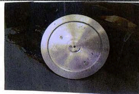
This picture is showing the machining done on the displacer.
