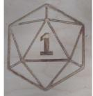
Carve two also failed, I thought the cleanup tool this time was 2mm but didn't check and the student before me had done something weird to the machine. This was a total waste of my time. I finally got a small sample done at 2mm and decided for future prints to increase both, along with increasing the size and decreasing the inputted size of the cleanup tool to 1.5mm
