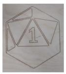
I set the diameter to 1.5 for carve three. It was working great but half of the way through the first carve a communication error occurred between the laptop running the routing software and the CNC machine. Normally when this happens the software manages to restart and simply continue from where it stopped. This time however, it didn't restart properly and instead moved to the wrong part of the print. I quickly shut it down to avoid mess and it compounds into bigger errors.
