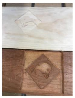
I have inspected the piece and it appears to have been routed properly. There are no blemishes or imperfections, and the design is well defined. On the trial piece the inlay design had some glue residue left over, this was because I didn't run it under the belt sander enough. To make sure that this didn't happen again, I made sure to run it under the belt sander until there was no residue left.
