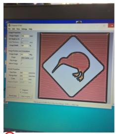
After drawing the design in Onshape and exporting it as a CNC compatible DXF file I opened it in an engraving and cutting programme to set the specifications of the engraving and cutting. The engraving programme allowed me to set the depth of cut (because the router uses a tapered bit that also controlled the width of the cut) and the feed rate.
