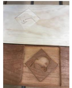
I have inspected the piece and it appears to have been routed properly. There are no blemishes or imperfections, and the design is well defined. On the trial piece the inlay design had some glue residue left over, this was because I didn't run it under the belt sander enough. To make sure that this didn't happen again, I made sure to run it under the belt sander until there was no residue left.
