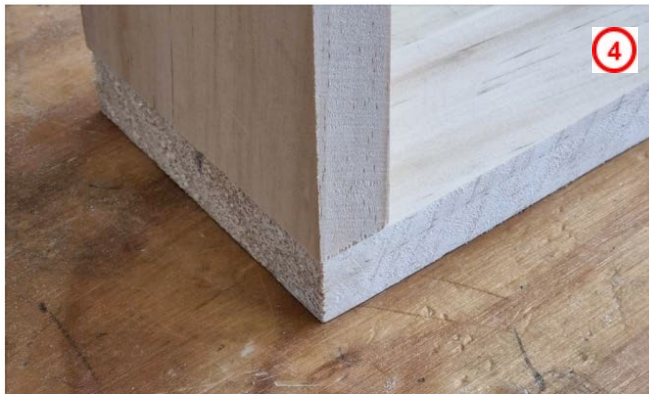
After trialing the biscuit joint I have decided that this is a good joint to use as I found it fairly fast to construct and with the use of glue and clamps this will make the joint very strong.
