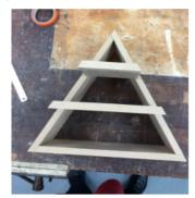
In this photo, we can see that we are doing a test cut for the housing joint to make sure that when we do the cut on the correct piece of wood it would be perfect. This took many adjustments to the table saw so that we could get the correct angle for the housing joint. We did end up getting it to the correct angle which was 30 degrees. My teacher helped with this for safety reasons
