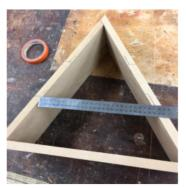
In this photo I am double checking that my housing joint cuts are going to be cut at the correct length. In this photo we can see that it is a 270mm gap for my shelf to go. This was put here because I needed the bottom shelf to be the biggest so that I could fit the biggest objects in. I made clear marks so that I knew where I needed to chisel out the gap for the housing joint.
