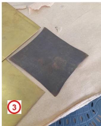
Preparing the brass for working. I measured out the sizes a few millimeters larger than needed to account for error, and cut them into a single square which would waste the least material. I cut it out with bench shear in the corner so i could get it against the edge which would tessellate better. Before rolling out, I cleaned the rollers from iron rust which would dirty the piece and could react in the pickle to form a pink metal layer. Before rolling I needed to aneel it to make it more malleable which would decrease the amount of rolling I would have to do. I rolled out so that I could get more out of the material to save cost and make it thinner which would look nicer/ be less clunky, would be easier to work and dome using the doming tool.
